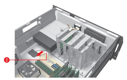
Figure 8. Removing the CD/DVD Power Connector
